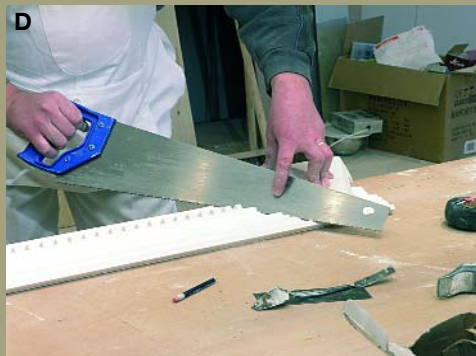
D With the saw blade resting on the mitre guide the cut can then be made
