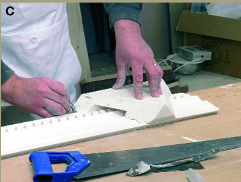
C Using the mitre guide, check that the cut leaves the pattern required
